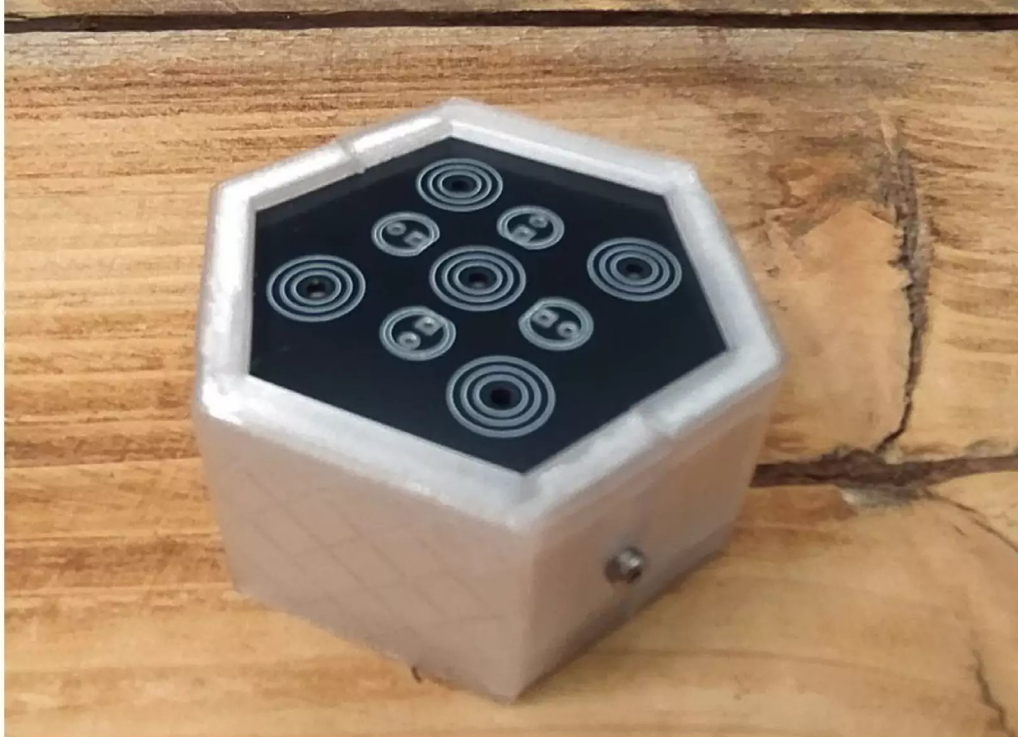
▲ Figure 9: A completed DIY enclosure with PCB front and rear panels; it would be simple to extend the case length in FreeCAD for larger projects
