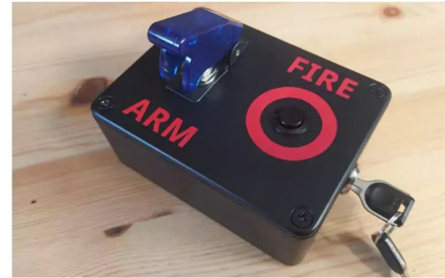
▼ Figure 6: Using a vinyl cutter can be an attractive way to make durable decals for an enclosure panel
