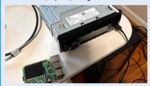
Adam's version of iAP2 enabling his car stereo to communicate with Raspberry Pi masquerading as an iPod was based on wiomic's iap2 (rpimag.co/iap2) and handles authentication, media controls, and metadata.
