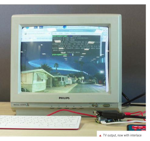
he very first Raspberry Pi had a composite video output, and all models with a 40-pin header have a display parallel interface (DPI) output. With some external components, DPI can be converted to VGA or RGB/SCART video. Those analogue interfaces are still in demand for retro media and gaming.
