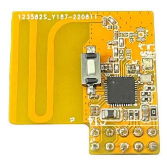
■ This mini GPIO module adds Z-Wave connectivity to Raspberry Pi
