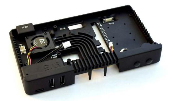
ports – including the GPIO header – are exposed within the housing for projects and there's a few millimetres of clearance for adding your own bits and pieces. Argon's signature daughterboard design is here too, with a PCB that plugs into the USB-C and HDMI ports of your Raspberry Pi, breaking them out to full-size HDMI and an additional two front-mounted USB-A connectors. Slotting it all together onto the plastic base creates a solid unit for your next project.
