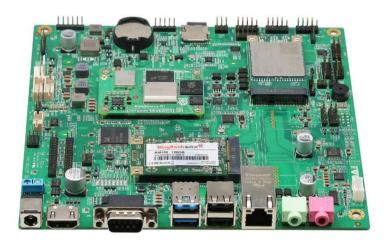
ased around a Raspberry Pi Compute Module 5 (CM5), EDATEC'S ED-SBC3300 range of industrial computers packs a whole load of processing power. The mini-ITX motherboard is identical to that of the earlier ED-SBC2300 range, but swaps out the CM4 for a CM5. Adherence to the mini-ITX form factor, with a 170×170mm footprint, means the motherboard can fit into any standard mini-ITX enclosure – or variants such as ATX and micro-ATX.
