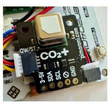
The all-important CO<sub>2</sub> sensor also provides temperature and humidity measurements
