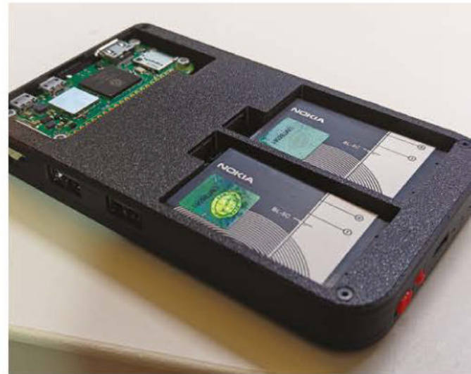
▼ The back of the device is just as smart-looking as the front, with compartments for Raspberry Pi Zero 2 W and the Nokia batteries
