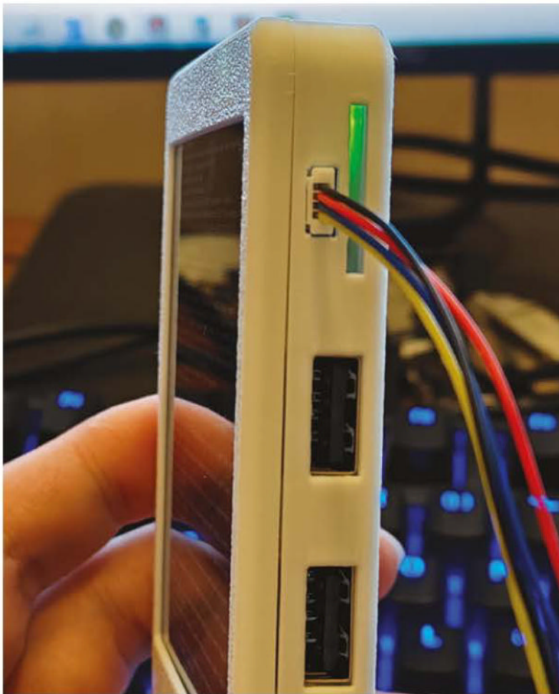
▲ A STEMMA QT port has been added, accessible from the right-hand side. It allows breakout boards and sensors to be connected
